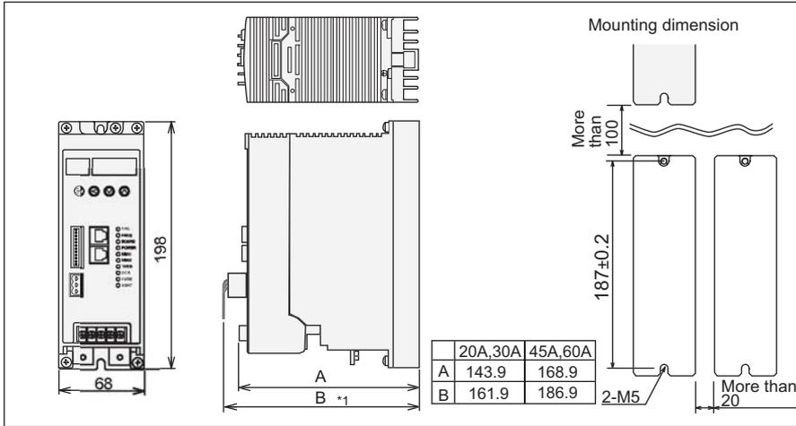
• Install the instrument as illustrated in the drawing to increase the cooling effect.
