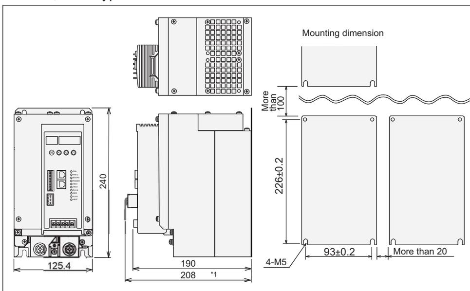
• The front of the instrument can be opened to allow replacement of the fast-blow fuse. When installing the instrument, leave enough space to allow the cover to be opened.
