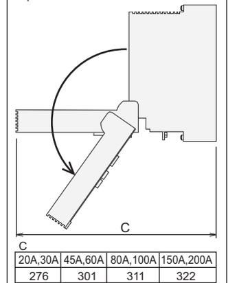
\*1 : Length includes that of an optional connector, but space for wiring to connector is not included.
